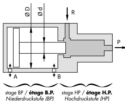
The multiplication coefficient is equal to the ratio of the surface areas of the BP cylinder and the HP piston: i.e.  $\frac{S}{s}$  or  $(\frac{D}{d})^2$ . In the rest position, the HP piston connects the receiver (port P) to a reservoir or external supply (port R). On the functioning of the cylinder, the HP piston seals the port R.
