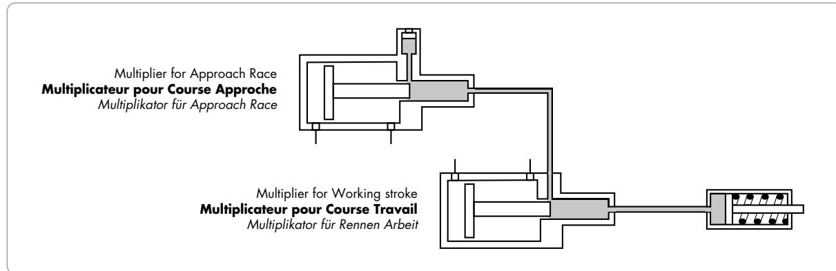
b) Using an exchanger for the approach and an MPA multiplicator for the working stroke.
