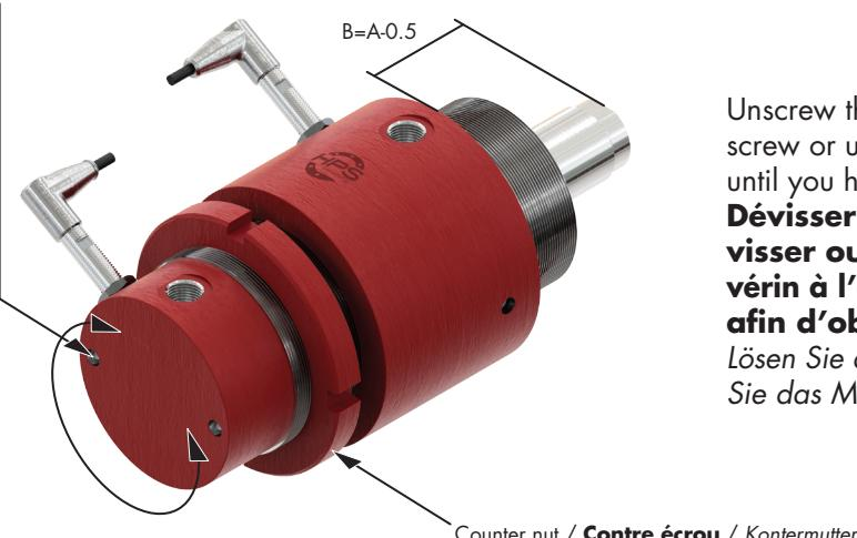
Unscrew the counter nut and then screw or unscrew the cylinder body until you have  $B=A-0.5$ .
